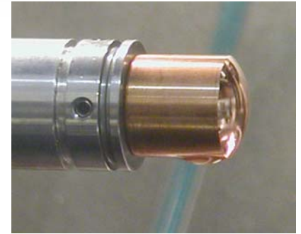
Copper sphere generated with spiral milling
