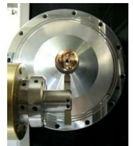
Copper sphere generated with spiral milling
