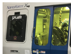
NXug with safety windows for laser assisted machining
